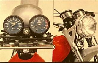
Enduro instrumentation includes speedometer, tachometer and resettable trip meter.
