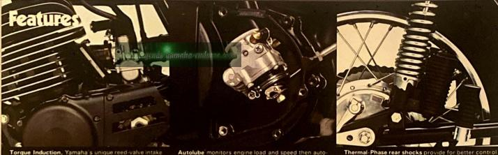
Torque Induction, Yamaha's unique reed-valve intake system, feeds theengine the exact mixture of fuel and air it needs. The result is more horsepower, particularly at low rpm's. Autolube monitors engine load and speed then automatically mixes oil and fuel accordingly. Constant flow adjustment to meet operating conditions helps extend engine life.
