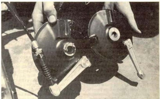
The stock front backing plate (left) must be machined down to slip in between the Simons sliders.
