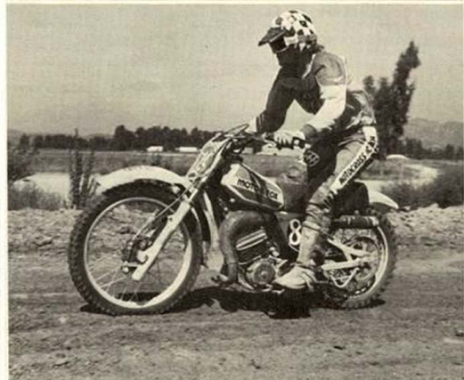
Off of Racing World's fastest jump the Moto-X Fox mono-mods soaked up the landing with ease. Check out the ground clearance, which means there is travel left.
