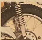
6 For maximum control and riding ease, the roar suspension is equipped with an adjustable 5-position system that allows the rider to change the tension of the rear shocks
