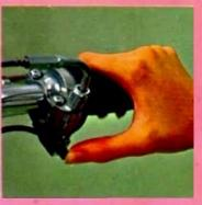
Engine can be easily stopped by simply pushing the button located conveniently near the right thumb. Safety plus.
