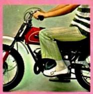
After starting, hold the clutch in and toe-shift. Then simply accelerate while releasing the clutch.
