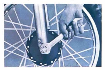
c) Remove the front axle by simultaneously twisting and pulling out on the axle.
