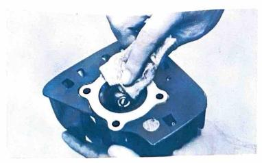
Bring the piston up to the very top and use the same scraping tool to remove the carbon from the top of the piston. Blow off as much of the loosened carbon as possible, then use the solvent soaked rag to pick up as much of the rest as possible.
