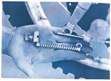
b) Remove the cotter pin and rear wheel shaft nut.
