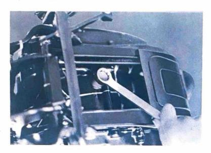
\*To drain the gear oil, the engine should be warmed up for 2 to 3 minutes. Then remove the oil drain plug from the crnakcase bottom, and the oil can readity be drained off.
