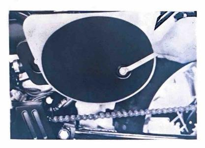
b) Remove the Oil tank and cleaner case cap.
