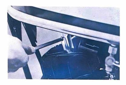
The plug can be taken out to be cleaned and gapped. As long as deposit built-up on the insulator is not extreme, you can use a spark plug cleaner to quickly remove the deposits. Use a wire type feeler gauge to set the electrode gap at 0.020"—0.024" (0.5mm—0.6mm).
