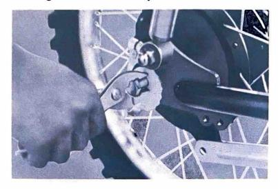
e) Lean the machine to the left and remove the rear wheel assembly.
