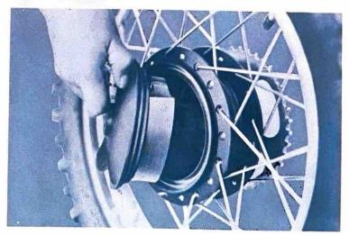
The brake plate carries both brake shoes. They can be left in place on the brake plate for measurement, or they can be lifted off for replacement or maintenance. The two brake shoes are held in place by two springs.
