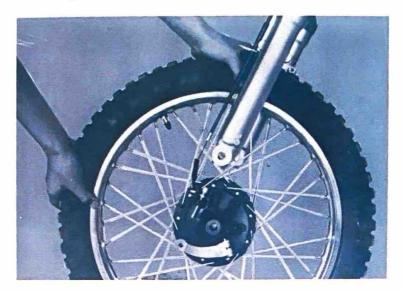
The brake plate can now be easily slipped out of the front wheel hub. The brake plate carries both brake shoes. They can be left in place on the brake plate for measurement, or they can be lifted off for replacement or maintenance. The two brake shoes are held in place by a spring. This spring holds the two shoes to the brake actuating cam.
