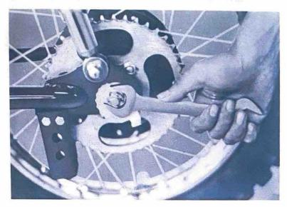
c) Push out the rear wheel shaft by striking it with a plastic tipped hammer.
