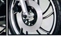
The wheels are YAMAHA Italic design, cast in alloy and finished in silver and matt black. The brakes are single disc front and waterproof, dustproof drum rear.
