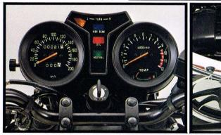
Instrumentation is comprehensive and includes sports tachometer and full range of warning lights. Self-cancelling indicators are fitted as standard.
