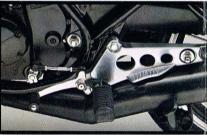
Cast aluminium plates act both as heel stoppers and to protect legs from the high-rise mufflers.
