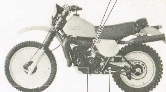
Shift pedal Ratcheting type 6-speed transmission (1T250F)
