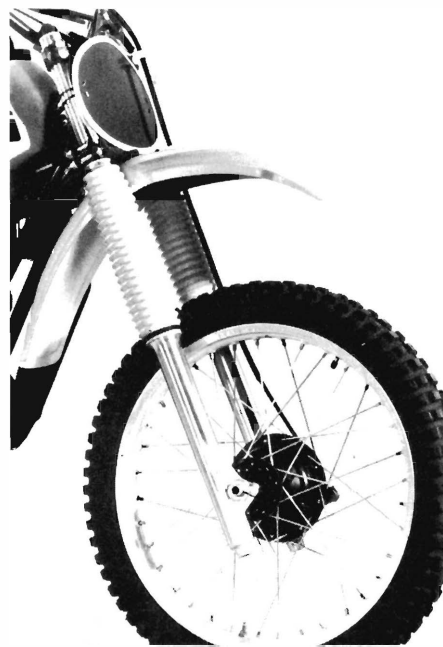
Magnesium and plastic has been used extensively to keep the Yamaha's weight competitive at 229 pounds.
