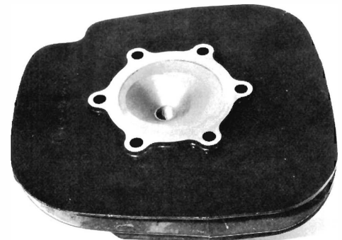
Yamaha's die-cast aluminum head has a new polyspheric combustion chamber dome and virtually no squish effect.
