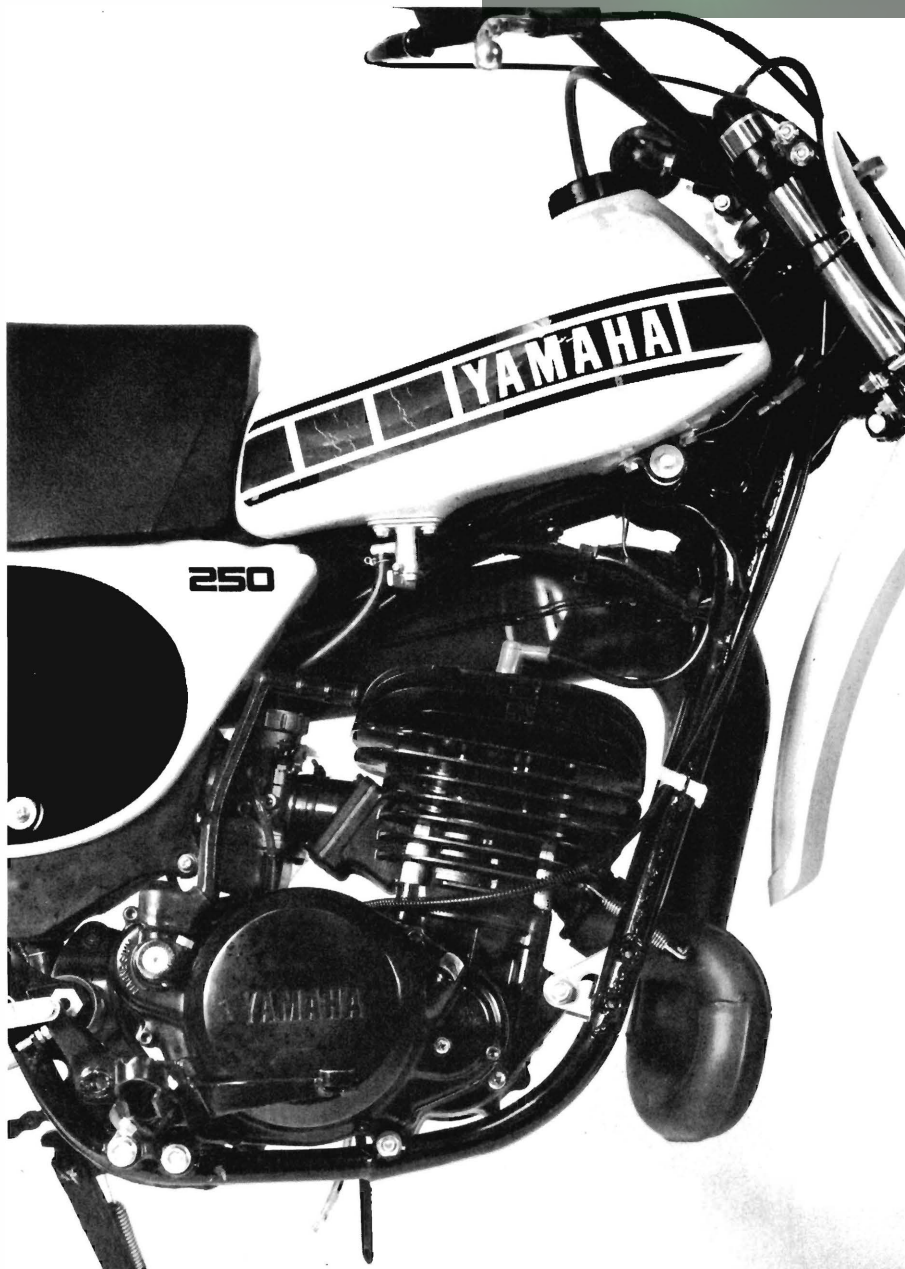
Magnesium and plastic has been used extensively to keep the Yamaha's weight competitive at 229 pounds.
