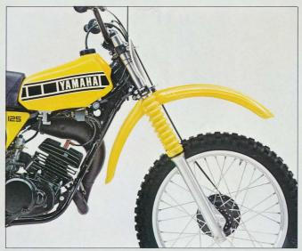
The leading axle fork design and lightweight front hub provide for quick, precise steering.
