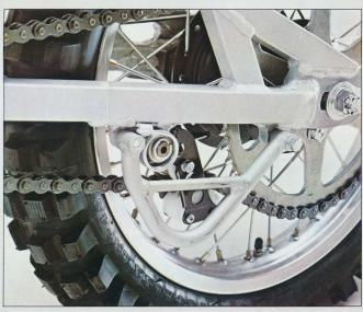
Long-travel suspension requires a chain tensioner. The improved design on the new YZ125 keeps the proper tension and reduces chain snap.
