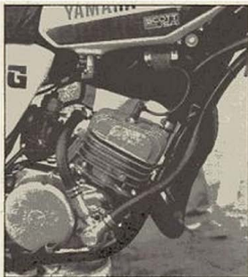
The aluminum alloy cylinder is a sandwich of water and chrome. The three hoses aren't the plumber's nightmare they seem to be.
