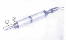
B.A.S.S. control cable smooth movement unsmooth movement→Repair or replace,
