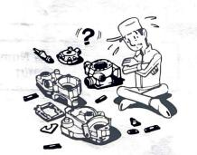
During the machine disassembly, clean all parts and place them in trays in the order of disassembly. This will speed up assembly time and help assure that all parts are correctly reinstalled.
