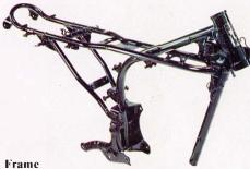
Utilizing the experience gained from the world's most demanding motocross tracks, YAMAHA has developed a lightweight, tubular-steel, single-down-tube frame that is able to give the machine an overall lower center of gravity for better maneuverability. This high-tensile-strength steel frame is designed to withstand the stresses and strains which are absorbed from the roughest of roads in order to assure long-term durability and stability.
