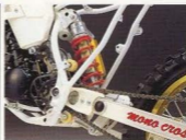
Suspension features an improved lever ratio and rear-suspension adjustability.
