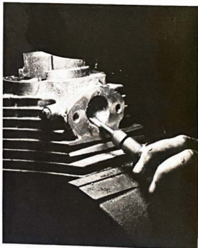
8. With the larger carburetor it will be necessary to open up the intake to match the new manifold or carburetor bore size. Try to be as careful and workmanlike as possible.
