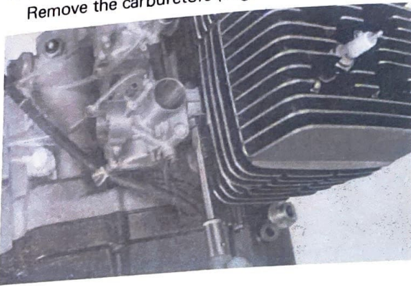
Fig. 4-2-1 Remove the nuts on the four cylinder stud bolts, (Fig. 4-2-2) then remove the cylinder head and cylinder head gasket. (Fig. 4-2-3)
