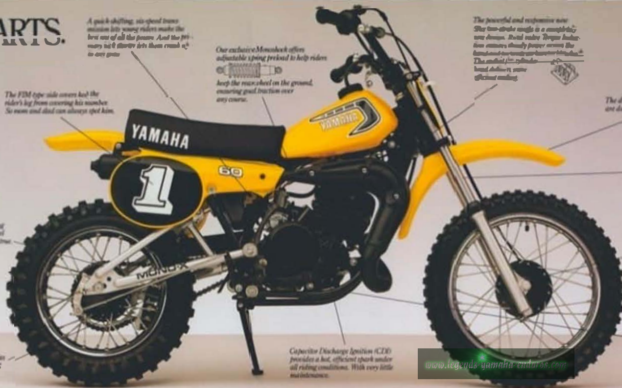
This year all the rugged features are built around a strong, lightweight single-down-tube tubular steel frame, just like our bigger YZ's.
