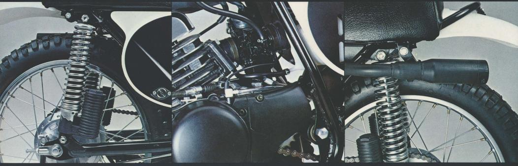
Thermal-Phase rear shocks have built-in oil coolers to prevent overheating, no matter how hard or long you ride. **Torque Induction**, Yamaha's unique intake system, utilizes a reed valve to feed the engine the exact amount of fuel and air it needs. The result is more horsepower, particularly at low rpm's.
