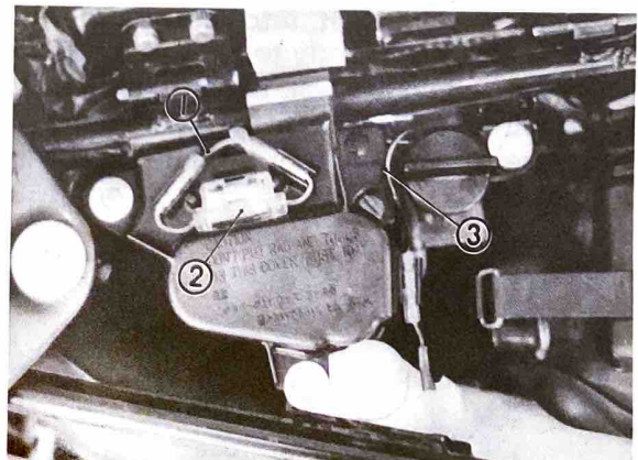
1. Positive lead wire 2. Fuse 3. Negative lead wire
