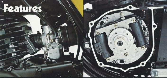
**Torque Induction**, Yamaha's unique reed-valve intake system, feeds the engine the exact mixture of fuel and air it needs. The result is more horsepower, particularly at low rpm's.
