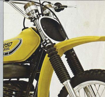
Yamaha's exclusive air cushioned front forks soak up sharp jolts without bottoming. Lightweight alloy rims and conical hubs minimize unsprung weight.
