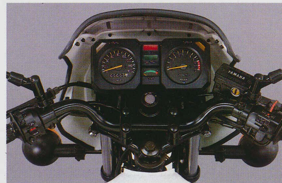
Speedometer, tachometer, temperature gauge, warning lights — the RD125LC is equipped with a full range of accurate, easy-to-read instruments. The ignition switch incorporates a safety steering lock position.
