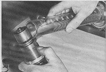
About 50cc of hydraulic fluid are poured into cylinder before piston slides completely in. This is 20w Lubritech fork oil.
