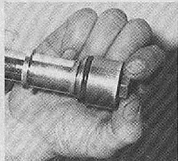
Nut holds piston in place, allows clearance for washer and wafer spring which act as one-way valve.
