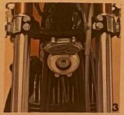
3. Hydraulic Disc dampener for better handling on and off the road. It consists of an oil reservoir and a paddle in the steering column. When the handlebars are turned, the paddle works against the oil, dampening the left and right travel. Ideal for dirt riding, since it prevents stones and ruts from radically deflecting the front wheel,
