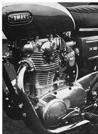
[4] A 653cc ohc aluminum twin cylinder engine is fitted with a couple of Solex type SU carburetors to deliver exclusive steadfast performance through a 5-speed gearbox.
