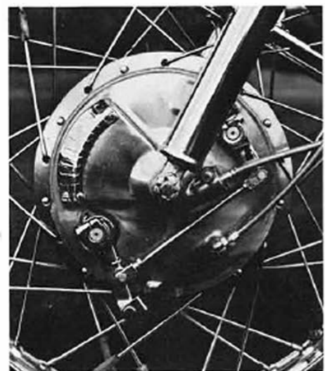
A cap-fitted from double leading-shoe brake is so powerful.
