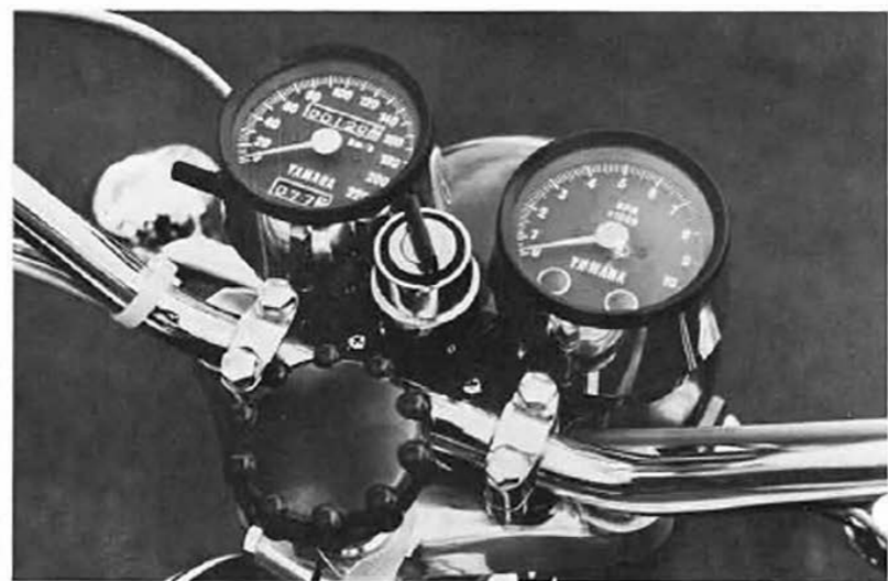
Newly designed speedometer (left), tachometer (right) and ignition key (center).
