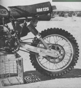
The 17½-inch Fox Airshox and the special aluminum swingarm offer 10½ inches of rear wheel travel.
