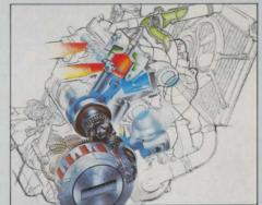
Liquid cooled 492cc V-4 two-stroke produces outstanding horsepower. Combined with an unprecedented power band, thanks to electronically controlled Yamaha Power Valve System (YPVS). Four centrally mounted 26mm carburetors supply the 50 degree V-4 through reed valve Torque Induction System. Double lubrication system teams updated Autolube and revresponsive auxiliary pump that prevents lube starvation during down shifts.
