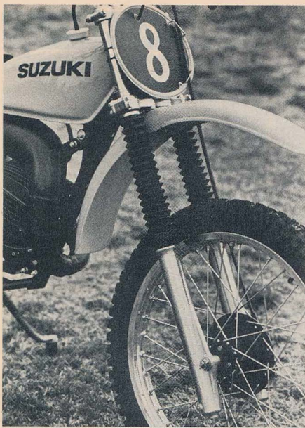
231mm of travel with ten-pound springs and air on top. We hope to see something very similar to these on the C model 250 and 370.
