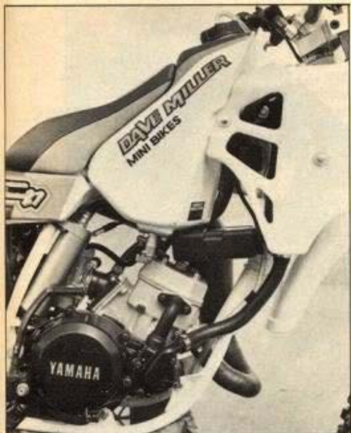
An aluminum "works-style" tank matched to a side-mount radiator give the C-27 its distinctive factory look.
