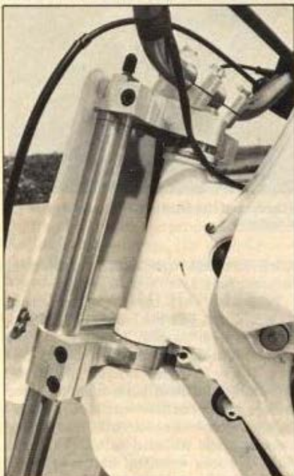
"Lowhang" triple clamps are mounted to CR80 forks up front. Upside-down forks are planned for the future.
