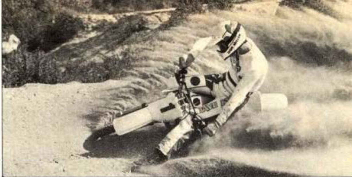
With the radiator weight off the front forks, handling through corners is first-rate.
