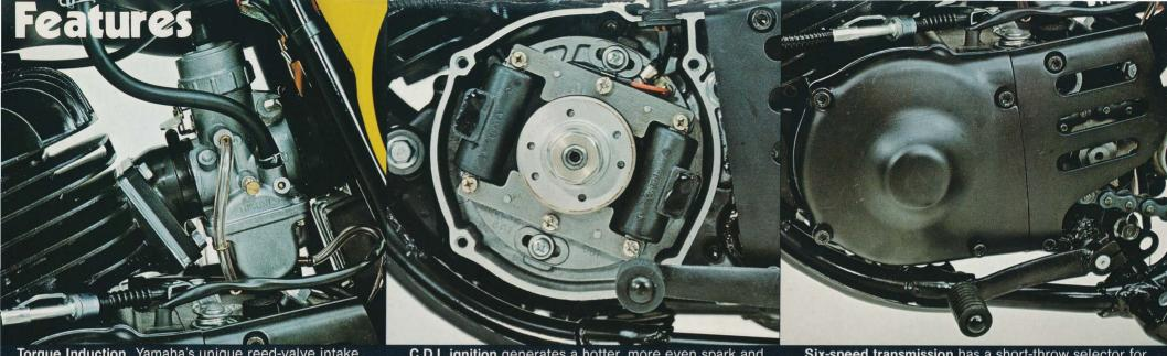
**Torque Induction**, Yamaha's unique reed-valve intake system, feeds the engine the exact mixture of fuel and air it needs. The result is more horsepower, particularly at low rpm's.
