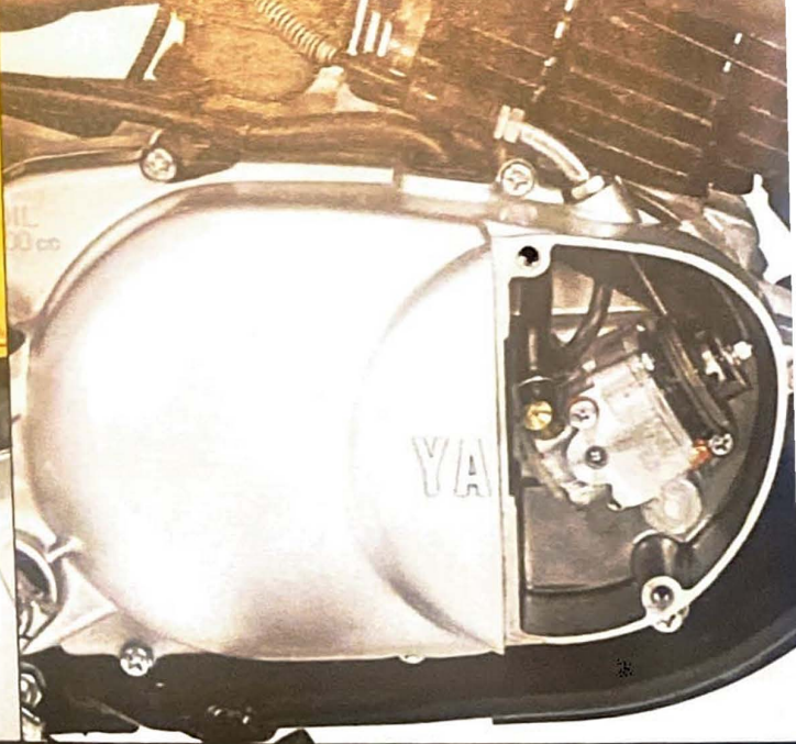
Autolube , a feature on most Yamaha two-stroke engines, automatically adjusts the flow of oil to engine load and speed, helping to extend engine life. And eliminating premixing.
