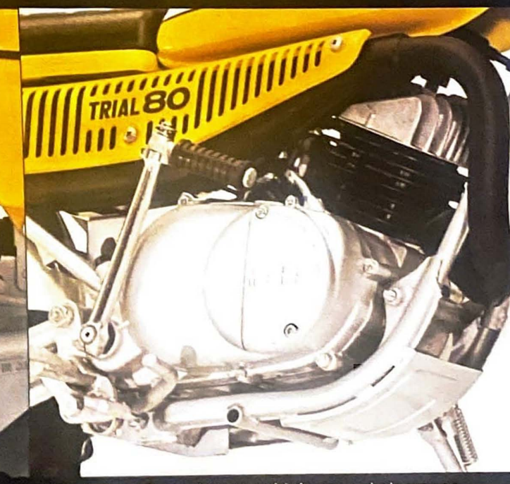
Trials type frame has very high ground clearance, yet, because center of gravity is still relatively low, the TY80 is easy to balance, even at very low speeds.
