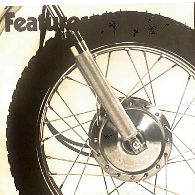
Large diameter front brake is water, dust, and fade-resistant. Long-travel front forks will soak up the hardest jolts and resist bottoming.
