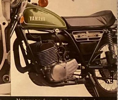
Torque Induction; Yamaha's unique intake system, utilizes a reed valve to feed the engine the exact amount of fuel and air it needs. The result is that horsepower is increased, particularly at low rpm's. C.D.I. ignition system produces a hotter, more consistent spark at all engine speeds, and virtually eliminates spark plug fouling. It also eliminates all the problems that go along with conventional breaker points.
