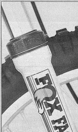
The new Fox Forx sport giant 44mm stanchion tubes and forged aluminum triple clamps and sliders.
