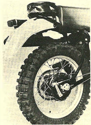
Subtleties abound: the brake rod routes over swing arm; removable pins let rear wheel pull straight out.
