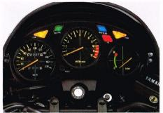
New, triple-meter instrument console features the central tachometer as its most prominent item. Speedometer, coolant temperature gauge and machine function warning lights are located on either side. All laid out in an easy-to-read, 'aircraft-style' format.
