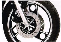
The twin front disc brakes and single rear unit are slotted to allow expansion without distortion from the heat of heavy use. Semimetallic friction pads ensure stopping power even in wet conditions, while opposed pistons in the rear brake caliper generate more braking force.
