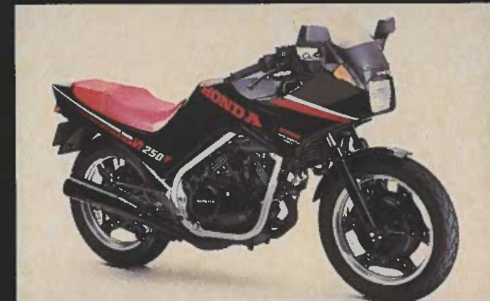
Japan's best-selling 250 is Honda's VT250F, a four-stroke, 90-degree V-Twin. The latest version makes an amazing 40 horsepower at a sky-high 12,500 rpm.
