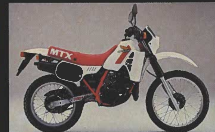
Enduro looks are offered by the Honda MTX200R, a liquid-cooled, ATAC-equipped dual-purpose bike. Despite the specs, it's more at home on the street than in the dirt.
