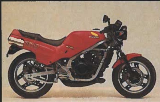
Steel-framed and unfaired, the Honda NS250F is cousin to the NS250R. Both use the same engine, but the F is $500 cheaper.
