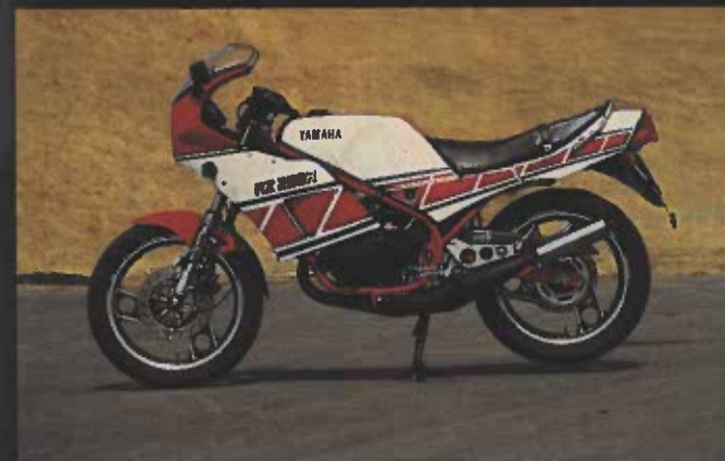
A frame-mounted fairing and a smaller engine distinguish Yamaha's RZ250R from the U.S. RZ350. Expect the new fairing in this country soon.
