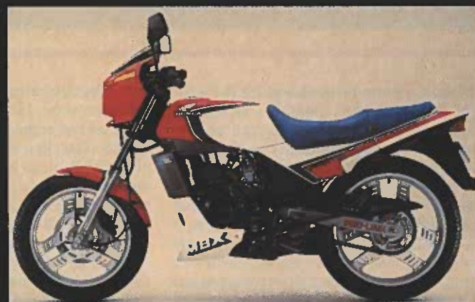
Honda builds two-stroke streetbikes for the very competitive Japanese market. This one is the MBX125, a 125cc Single that puts out more than 20 horsepower.
