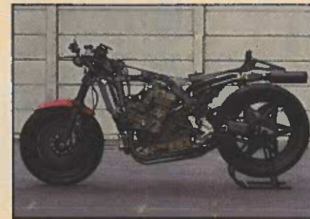
Carbon-fiber frame on HRC's NR500 showbike is for looking, not riding.
