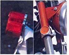
New Safety Features: Spot reflectors on both sides of the front fork for added safety. Tail light is activated by using front brake. Flasher lamps are available at option. All these meet federal safety standards.
