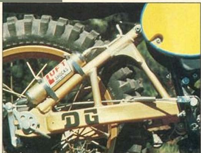
A Luft modified shock and reservoir, combined with an aluminum swing arm, helps transform the little IT into a fine handling machine. K190 has grip like super glue.
