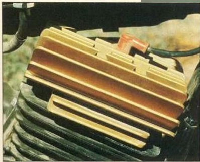
Radial finned aluminum head cools better than stock and increases compression slightly.
