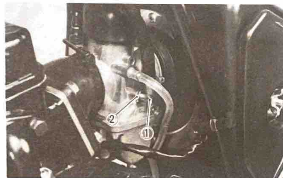
1. Throttle stop screw 2. Lock nut
