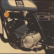
Motocross-type frame cradies the engine lower, has lower center of gravity for better handling. This frame design, adapted from the highly successful Yamaha motocrossers, also flexes less, for surer tractions.
