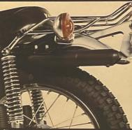
Silencer and multifer design cut down noise without cutting down power. Over-the-top exhaust and expansion chamber for better road clearance, less chance of burns.
