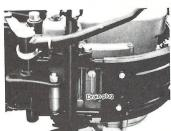
After draining the oil, fully tighten the oil drain bolt, and fill with new oil to the specified level.
