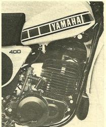
The YZ400E has a new box-section swing arm and a tubular chain guide. The rear structure is stiffer and lighter than the D-type. The engine has remained the same but is still strong enough to win.
