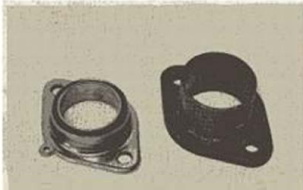
For more efficient breathing, the larger exhaust flange at right is used in conjunction with the triple-staged downswapt pipe.
