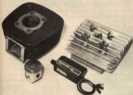
These parts with a 32mm Mikuni and downpipe will help any YZ125 become a potential threat in local motocross.
