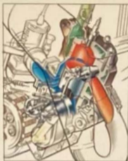
2-stroke, liquid-cooled, single
