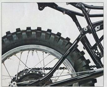
**De Carbon Monocross Suspension,** Yamaha's revolutionary suspension system, provides greater rear wheel travel for better control, more comfort and consistent traction over rough terrain.
