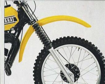
New Leading axle front forks are air cushioned with increased travel for soaking up bumps. Conical hubs help reduce unsprung weight. And lightweight polypropylene fenders are virtually unbreakable.
