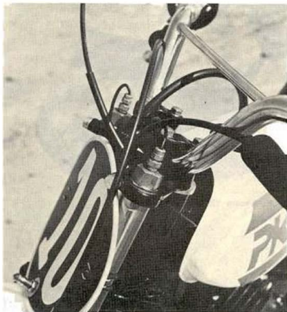
Forks are gas pressurized, but they run together.
