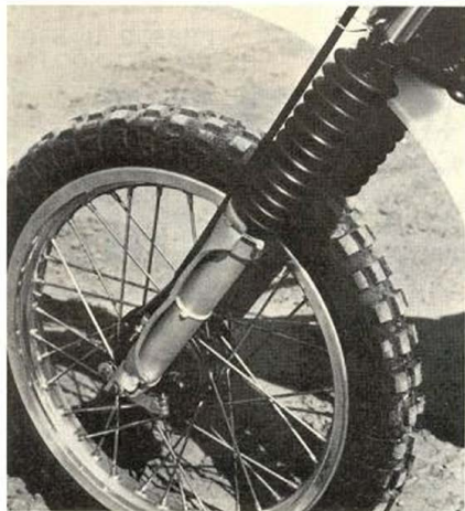
Forks are machined down so they look like they came off Hanna's factory Yamaha.
