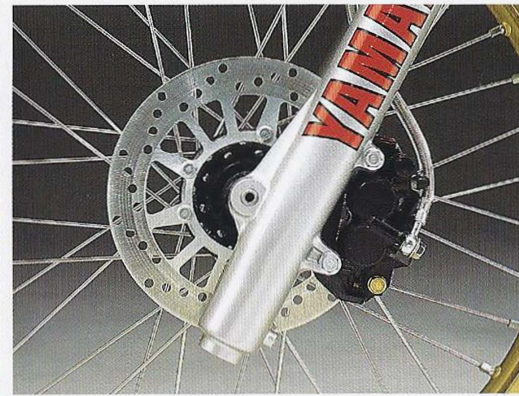
Up front you'll find a set of massive forks along with a 220mm steel disc.
