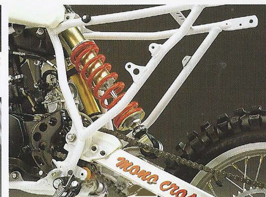
Our little YZ shares monocross suspension with our bigger YZ's.
