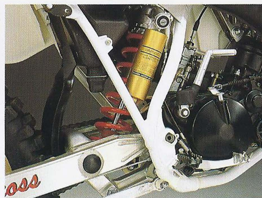
Brake Actuated Suspension System helps keep rear-wheel on track.
