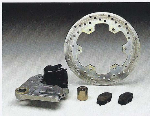
The rear disc is a whopping 220mm, mounted on a new, lighter hub.
