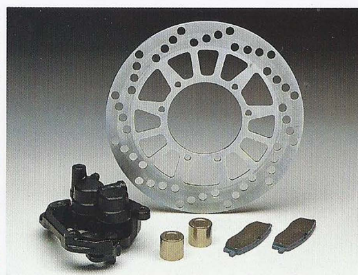
The carbon-steel drilled front disc has been beefed up to 230mm this year.
