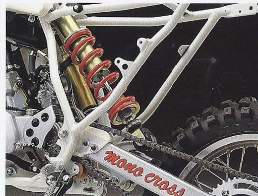
The little YZ's Monocross rear suspension is just like that of our bigger YZ's.
