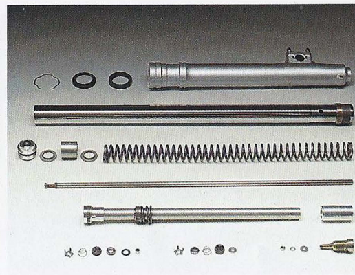
New cartridge forks offer more consistent rebound/compression damping.
