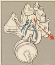
2-stroke, liquid-cooled, single
