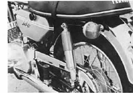
In rear cushion, spring pressure is freely adjustable in three stages.
