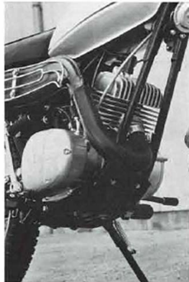
Impressively high ground clearance. Moreover, steel engine guard ensures safety in rough riding.
