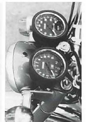
Main switch is placed in an easy-to-operate position. Light switches are gathered on left handle.
