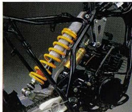
Yamaha's Monocross single shock suspension has been developed and proven on race winning YZ motocross bikes. It gives a true rising rate by virtue of a sophisticated linkage, allowing free movement over small bumps with more control when the terrain gets tougher. On the IT200, it features a remote reservoir, infinitely adjustable preload, and rebound and compression damping adjustments.
