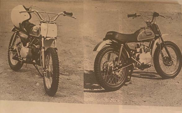
front forks contain oil, the only access plug for drainage purposes is on top of the fork tubes. And the ball-ended hand levers tend to break off rather than bend. But for a youngster, these are minor shortcomings.
